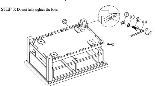
STEP 4: Using the Allen key (G) tighten all bolts
